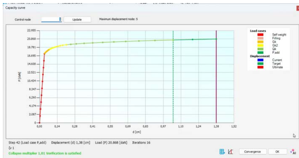
Fig. 23 - Capacity curve of the vault, or the graph that reports on the X-axis the displacement of a control node, which by default is the node that at the end of the calculation has a greater vertical displacement, and on the Y-axis the load applied to the vault in a progressive manner.
