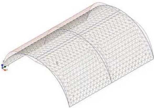
Fig. 18 - Three-dimensional visualization of the displacements of the mesh nodes of the turned surface after the analyses.
