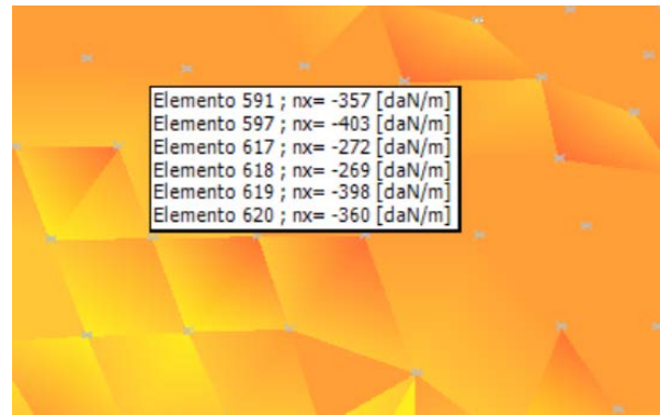
Fig. 25 - Viewing stress results by moving the mouse over the 3D surface
